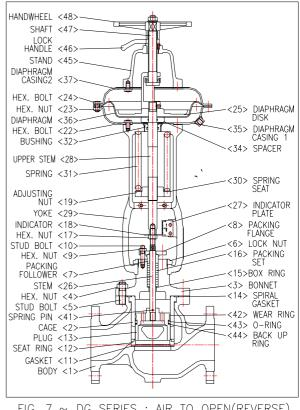
FIG. 7  $\sim$  DG SERIES : AIR TO OPEN(REVERSE) TYPE ACTUATOR AND VALVE BODY ASSEMBLY
