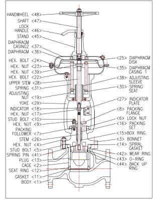
FIG. 6  $\sim$  DG SERIES : AIR TO CLOSE(DIRECT) TYPE ACTUATOR AND VALVE BODY ASSEMBLY
